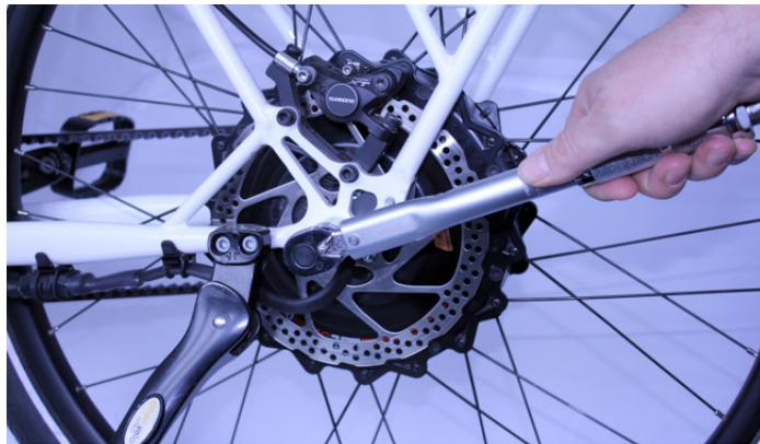
4. Tighten the torque arm bolts to the specified torque of 8-9 Nm to the frame.
