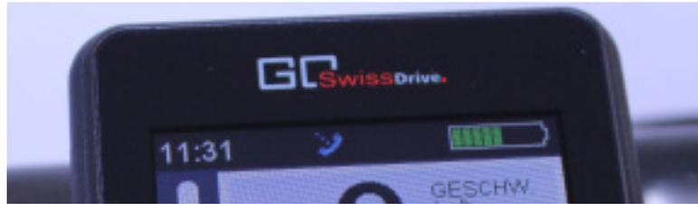
Fault: If a fault occurs in the GO SwissDrive drive system of the E-Bike, this is shown in the display. A pop-up appears (see chapter 7.2 "Warning notices") along with a fault symbol in the status line.
