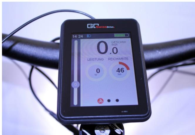
When the recommended gear change is activated, arrows on the right of the speed display indicate which speed should be selected. An up arrow is an indication by the system to shift to a higher speed using the bicycle's chain gears. If the arrow is pointing down, this is a recommendation by the system to select a lower speed.
