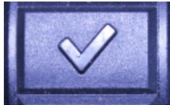
**[+]/[-] buttons:** The power assistance level of the GO SwissDrive drive system can be set with the [+]/[-] buttons. In the configuration menu, the [+]/[-] buttons are used to navigate between the individual menu items and change numeric values.
