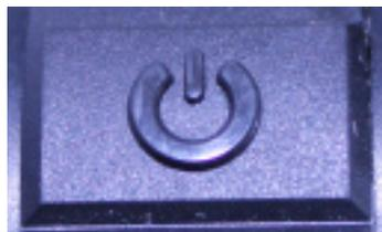
**[Confirm] button:** With the [confirm] button, various functions in the menu of the EVO operating element can be activated and deactivated. It is also possible to select and confirm settings in the configuration menu. The function of the [confirm] button here depends on the currently displayed menu.
