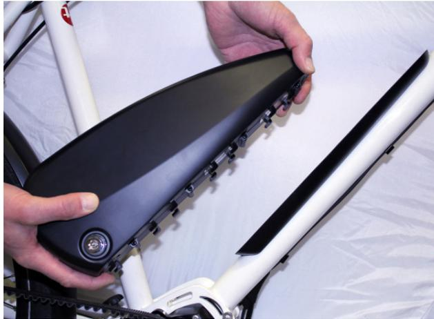
2. After removing the battery, switch the EVO operating element on and off again in order to completely de-energise the system. The rear wheel must be stationary when doing this.
