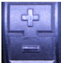
**[Next] button:** The [next] button is used to change between the individual menus of the EVO operating element. The order of the menus is predetermined and cannot be changed. It is possible, however, to deactivate individual menus in the settings. Deactivated menus are left out when the next one is selected.
