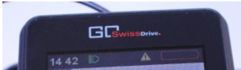
Battery charge level: The battery symbol on the right edge of the status line indicates the current charge level of the battery. The symbol has 9 bar segments with each bar representing 10% of the battery capacity. A detailed description of the display depending on the charge status can be found in the following table.
