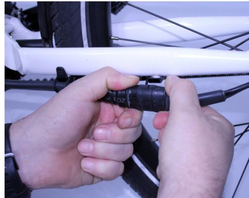
8. Finally, attach the cable with a cable tie or secure in the dedicated position on the frame. The cable should not protrude outwardly to the side nor interfere with the spokes of the rear wheel or rub against the motor.
