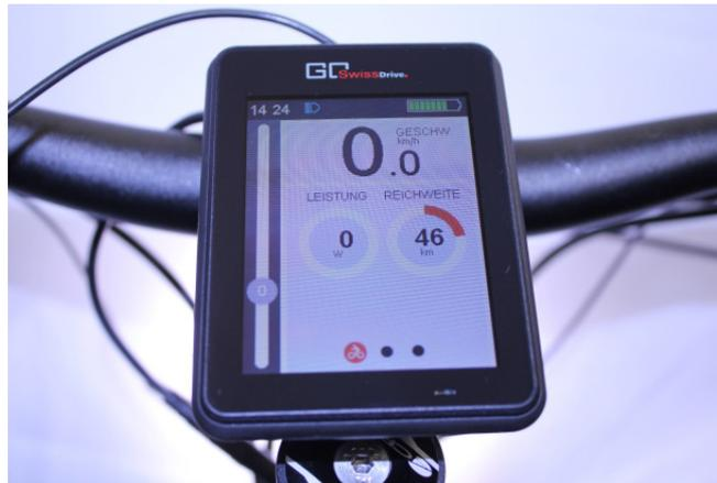
The status line provides a quick overview of the current system status by means of various symbols.
