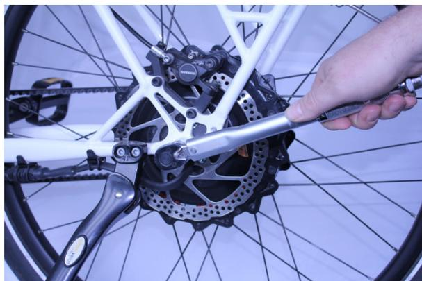
5. Now secure the torque arm to the frame and tighten the bolt, if present, to the prescribed torque of 8-9 Nm\*.
