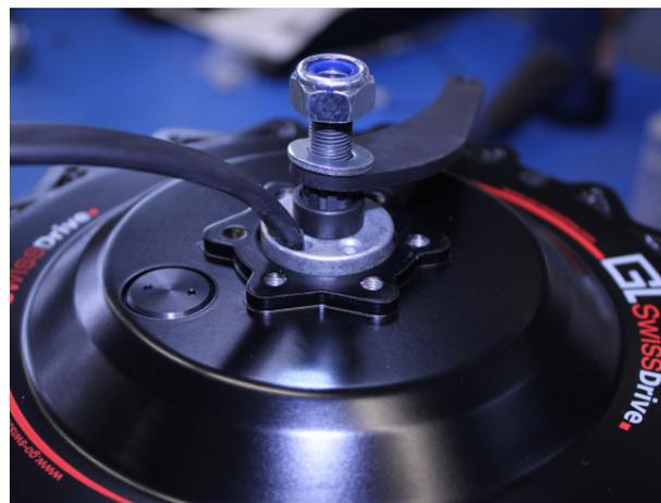
2. Then, unless already done, guide the quick release axle through the hollow axle of the rear wheel. Screw the counternut by hand 2-3 turns onto the thread of the clamping axle to ensure that there is sufficient clearance when installing.
